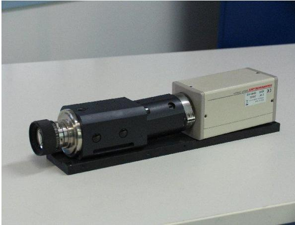
Attach the camera to the spectrograph as described in other documents. It is assumed here that the spectrograph is adjusted so that the spectral and spatial axes are orientated correctly to detector rows and columns.
