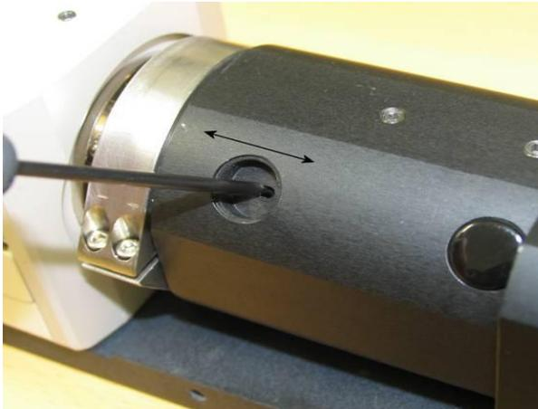
Adjust the back focal length of the spectrograph if needed. For this one should check the document "TN07\_Adjustment\_of\_the\_back\_focal\_length (BFL)"
