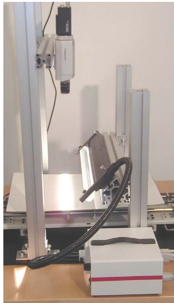
Figure 1. A typical spectral imaging setup with fiber optic lightline.
