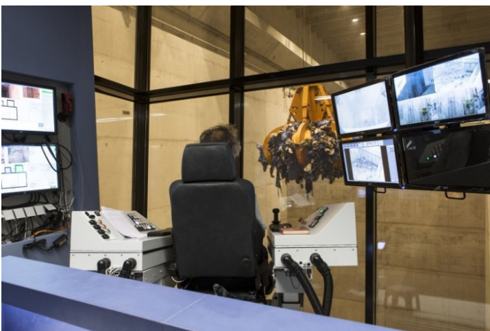
Fig. 3: In the crane cockpit, the crane operators have access to all central functions of the WASTE-SCAN infrared monitoring system at any time. For example, they can selectively control individual cameras manually from there.
