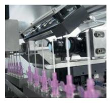
information can be fed back into the process to systematically rectify the problem at the point where it originates, resulting in increased system productivity and availability. Machine vision technology is unique in its ability to resolve the trade-off between raising quality and cutting costs. Examples abound in which machine vision does both jobs at the same time.
